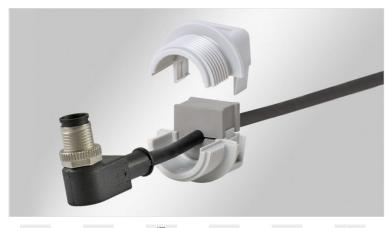
QVT is a circular split frame for quick and easy installation of pre-terminated cables or complete cable harnesses. But also electric, pneumatic or hydraulic lines without terminals or connectors as well as corrugated conduits can be easily routed and sealed with IP54. Because of its extremely compact design, the QVT range is especially suitable for small machines, devices and instruments.
